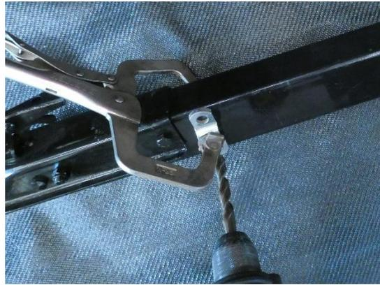
If mounting to a single tubular tongue drill all the way through the hole on the other side as shown below to assure the holes will align:
