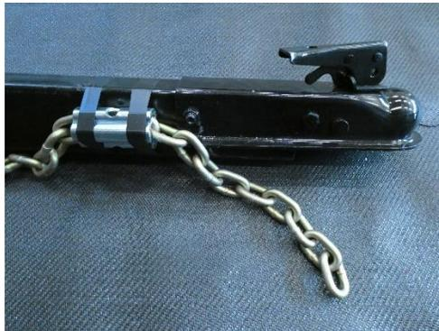
Mark or measure the position of the LinkLock™ sleeve on the tongue. Now Clamp the LinkLock clamp plate to one side of the tongue with the front edge at the same position as the front of the LinkLock™ sleeve was positioned as shown below. This will be used as a drill guide for drilling the two holes through one side of the tongue.
