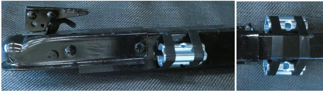
As shown below, insert the LinkLock™ pin into the hole in the sleeve to assure there is nothing blocking it from complete insertion. Do this on both sides as there may be interference on one side and not the other.
