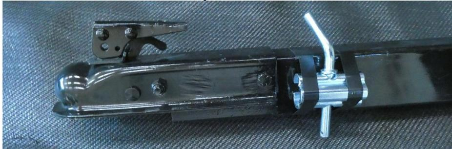
Next, insert the 5/16" safety chain with the chain link welds away from the tongue (it works better this way). Make sure the chain will slide smoothly back and forth through the LinkLock™ sleeve without anything blocking it.
